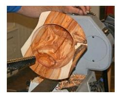
The part turned bowl was reversed onto the chuck and the thickness of the wings reduced further. He was careful to ensure the outer edge of the raised lip lined up with the outer edge of the underside of the bowl below the wings. Finishing cuts on the upper surface of the wings were taken with a scraper.
